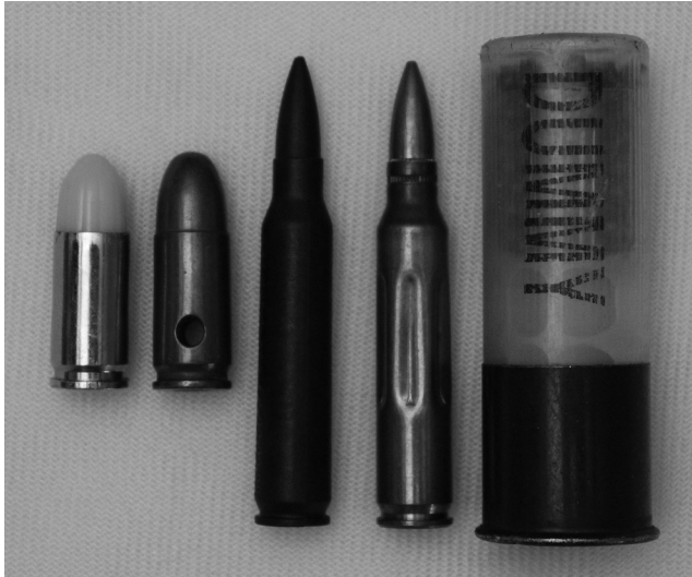
Figure 2.28 (See color insert.) Examples of various dummy, drilled, and inert cartridges (from left to right): safety orange marked 9×19mm, drilled casing 9×19mm, solid black plastic 5.56×45mm, corrugated casing 5.56×45mm, and a 12-gauge shell marked DUMMY. (Image from author's collection.)
